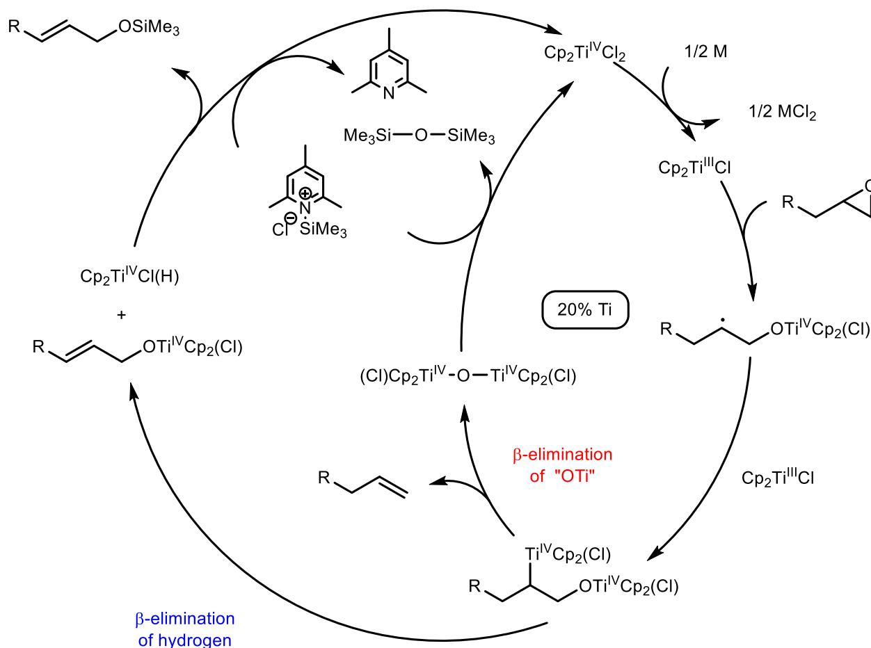
Catalytic  $\text{Cp}_2\text{TiCl}$ -mediated epoxide opening with use of  $\text{TMSCl}/2,4,6$ -collidine
